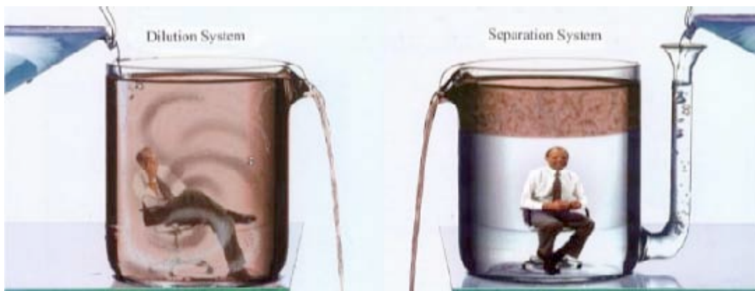
Figure 4: A metaphoric comparison between the so-called ‘dilution’ and the ‘separation’ systems of air ventilation. According to the image, the separation model is superior in that heated and ‘dirty’ air leaves the room at the top, while cold clean air enters from the bottom and is not circulation or ‘diluted’ with used air. Source: Kluske, 2009
