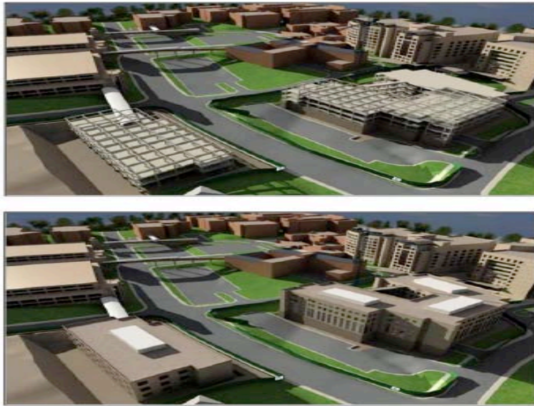
Figure 4: Using digital models the developers of a hospital project in Charlotte, North Carolina can plan their operations pre-construction, demonstrating not only what the hospital will look like in completion, but during construction and with scaffolding still in place. (Source: AutoDesk White Paper, 2005, 9).
